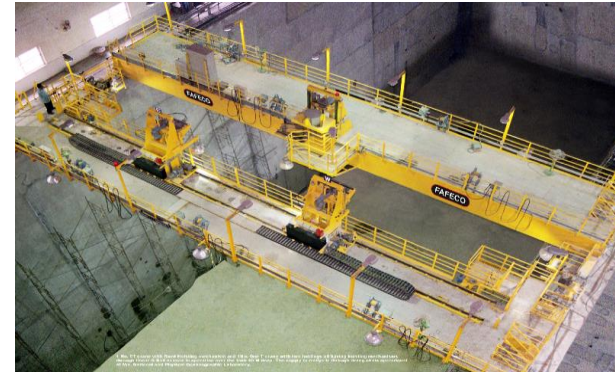
Rotating Beam Anti-sway Magnet Crane
